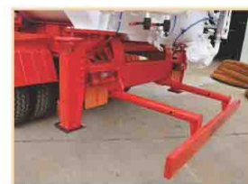
Sliding Type RUPD to Expand and retract
