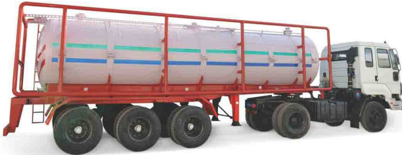
20 kl Chemical Tanker Made from Aluminum with Safety Frame
