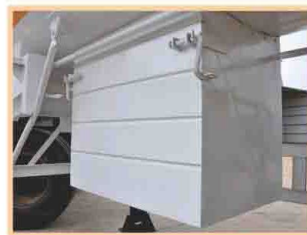
Valve Box with V Opening for Better Access of Valves
