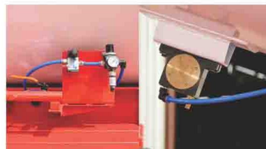
Pneumatic Vibrating Motor with Manual Operating Valve
