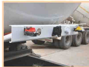
Broad mounting plate for ABS and Brake Coupling at front center of tank
