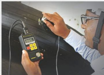
Ultra Sound Thickness Gauge
