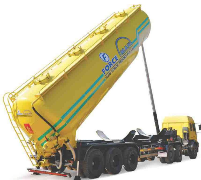
38 m3 Tipping Tanker with Hydraulic Stabilizing Jacks
