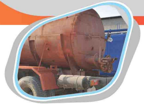
Jacketed Tank with Heating Tanker
