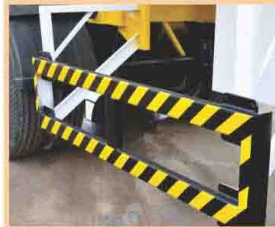
Hinged SUPD for hassle free operation of valves
