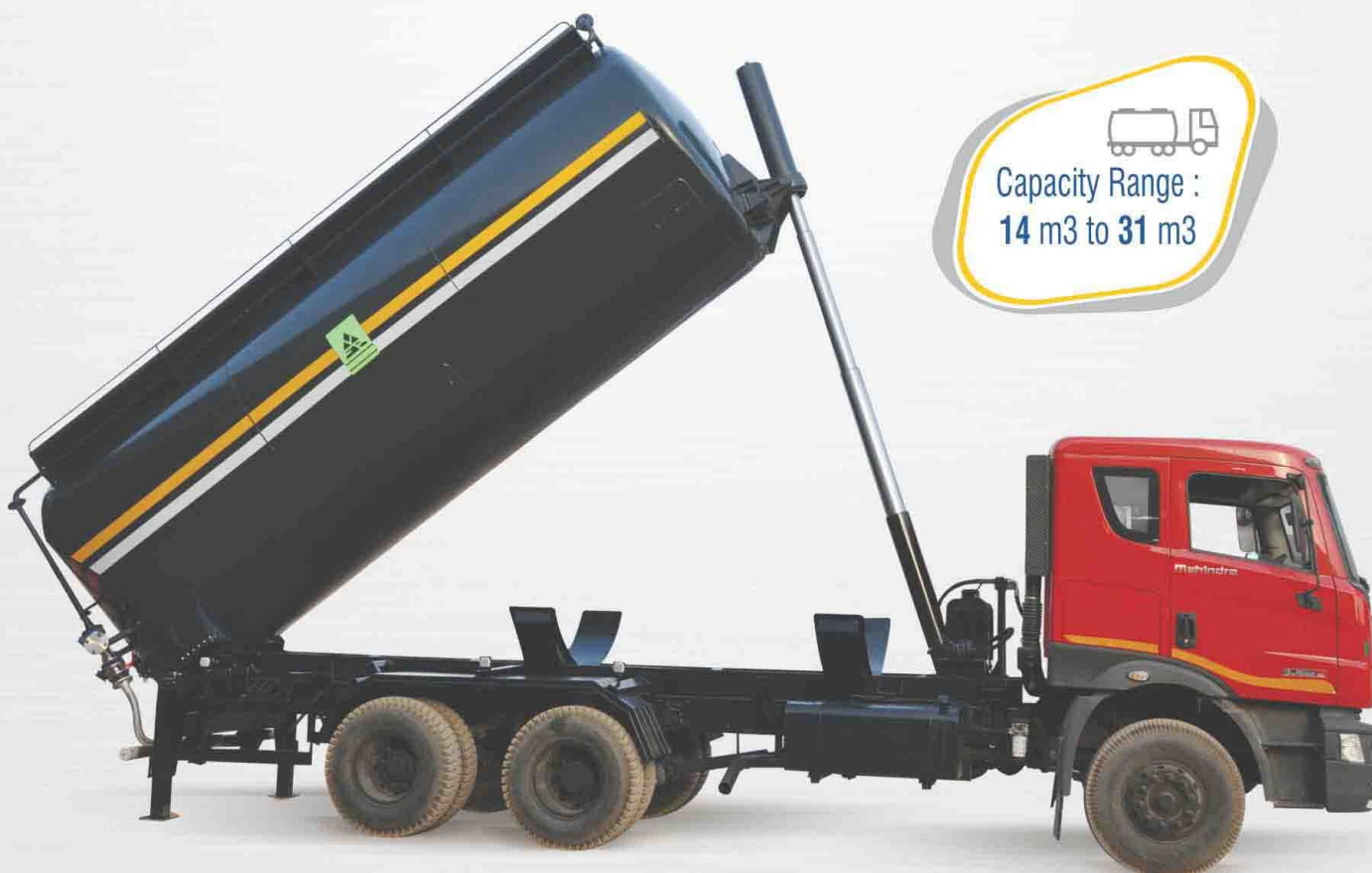
25 m3 Made from Aluminum for Flour
