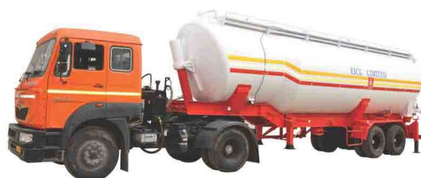
45 m3 with Pneumatic Vibrating Motor
