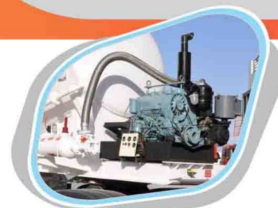
Compressor with Auxiliary Engine
